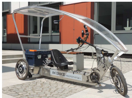
Example of the e-trike equipped with dedicated drives working in pedaling-by-wire (PBW) conception of control. Mechanics made by Agregaty Polska company
